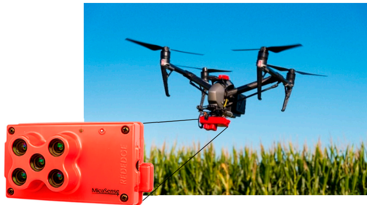
Figure 3. DJI Inspire 2 multi-rotor UAV with MicaSense® RedEdge® five-band multispectral sensor and downwelling light sensor. Inset image is a close up of the five-band multispectral sensor.
